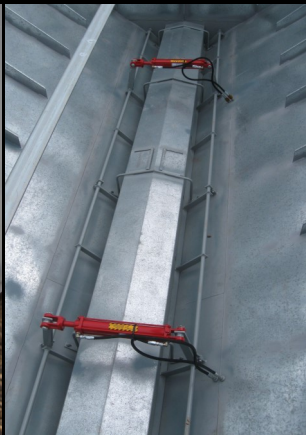
Hydraulic controlled shut off doors cover sweep flight
