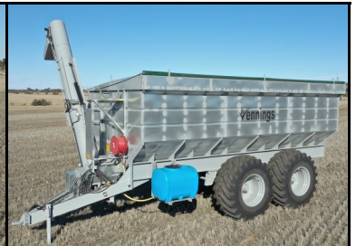
46 M 3 Approximately 33 Ton Bin with Springs, Steering & Brakes
