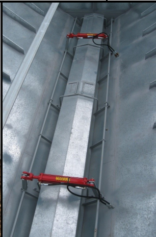
Hydraulic controlled shut off doors cover sweep flight
