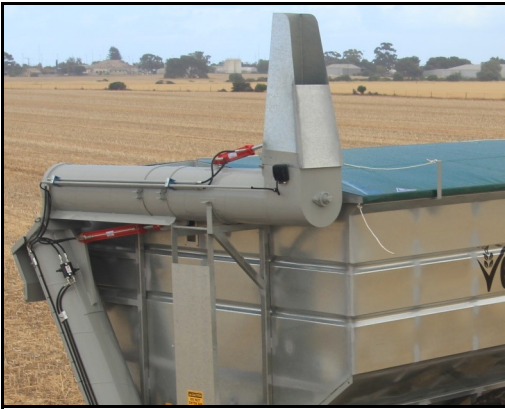
33 M 3 Bin with auger folded fitted with standard hydraulic folding discharge chute
