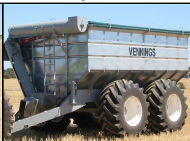
30 M 3 Approximately 25 Ton Bin Rocker & Steering Axle
