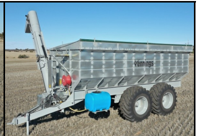
46 M 3 Approximately 33 Ton Bin with Springs, Steering & Brakes
