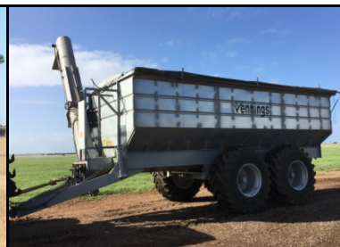
33 M 3 Approximately 28 Ton Bin With Springs, Steering & Brakes
