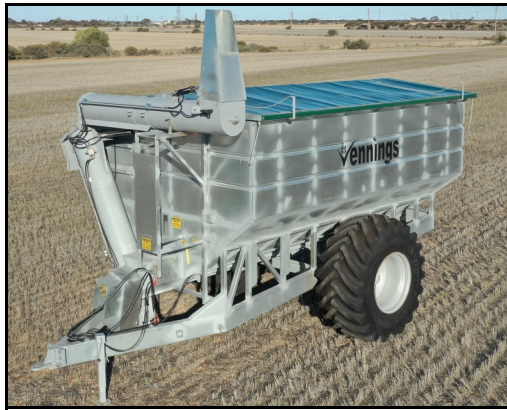
27 M 3 Bin with auger folded fitted with standard hydraulic folding discharge chute
