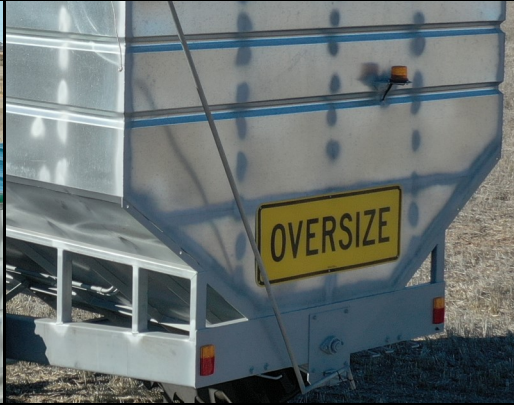
Bin fitted with LED Turning & Brake lights, Revolving Light and oversize sign
