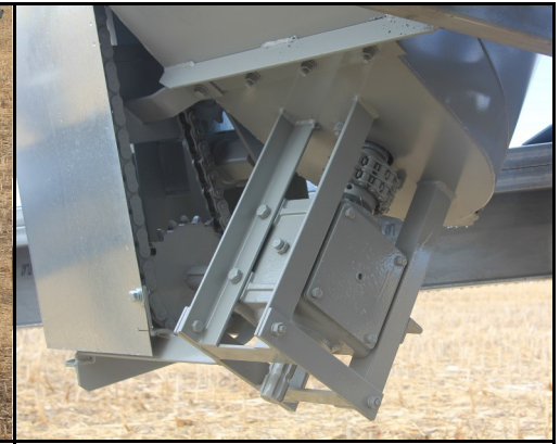
Heavy Duty Gearbox with 1" Drive Sprockets
