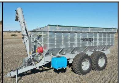
46 M 3 Approx. 33 Ton Bin with Springs, Steering & Brakes
