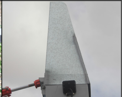
Hydraulic folding adjustable spout with 1200 lumen LED work light
