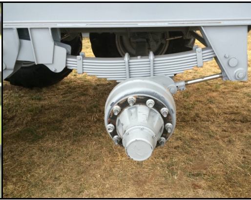
Fitted with Extra Heavy Duty 9 Leaf 100 x 16mm Sprung Pivoting Steering, Braked Axles
