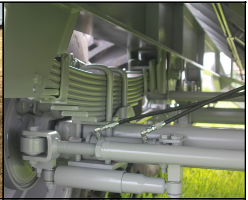
Hydraulic rams fitted to rear axle to allow bin to be reversed into sheds etc.
