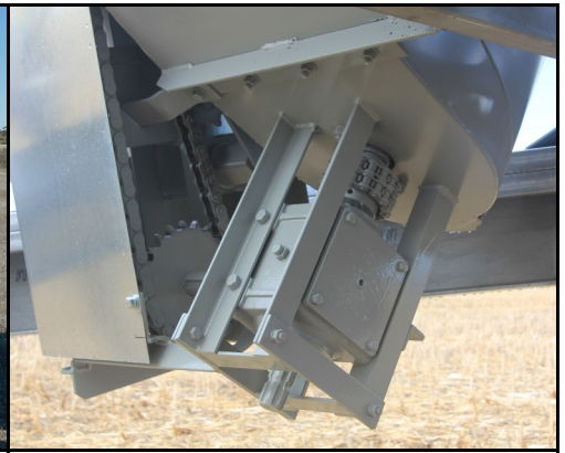
Heavy Duty Gearbox with 1" Drive Sprockets
