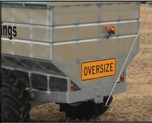
Bin fitted with LED Turning & Brake lights, Revolving Light and oversize sign
